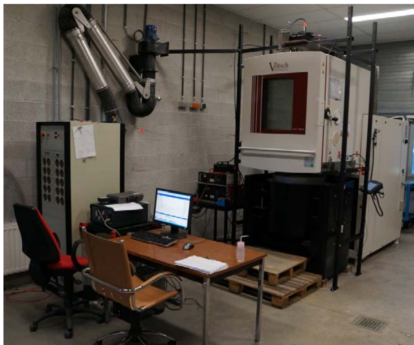
Figure 7: Climatic chamber (here, coupled with shaker 26 kN Ling A395)
