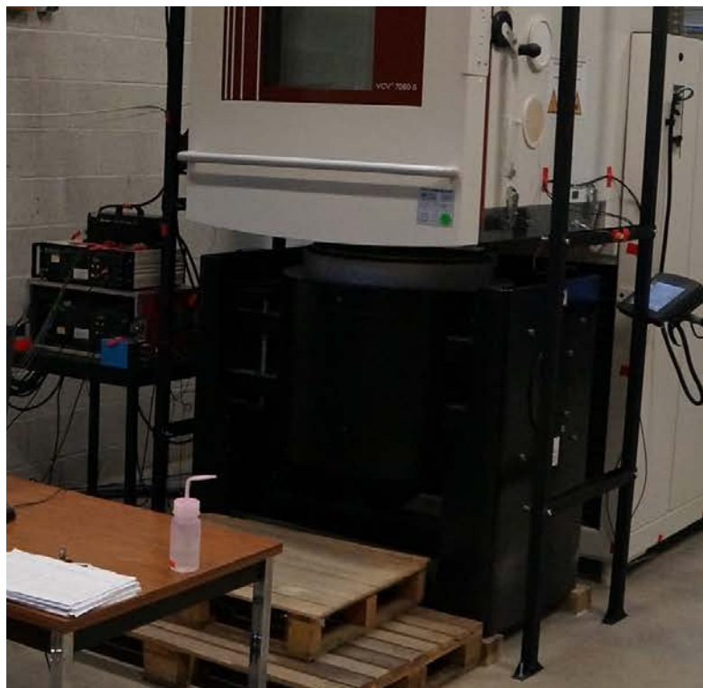
Figure 4: LE A395 (26 kN) (here coupled with climatic chamber).
