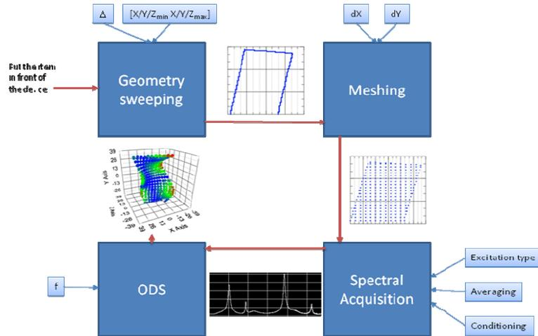
Figure 2 - Software architecture
